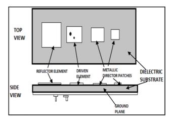
Figure 1: Microstrip Yagi-Uda Configuration
