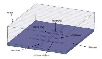
Figure 2: Antenna Design on HFSS Software
